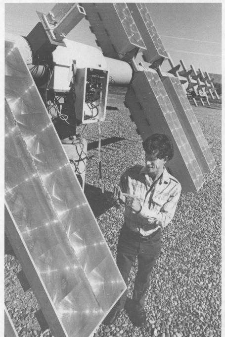
ALEX MAISH (6221) keys data into user-interface board to check the performance of the SolarTrak controller, an autonomous solar tracking system (in cubicle in center). The array tracks the sun in its path across the sky based on time readings and location rather than less-reliable sun sensor data. The system is being manufactured and marketed by three solar energy companies that have negotiated non-exclusive licensing agreements with Sandia. (Photo by Mark Poulsen,
